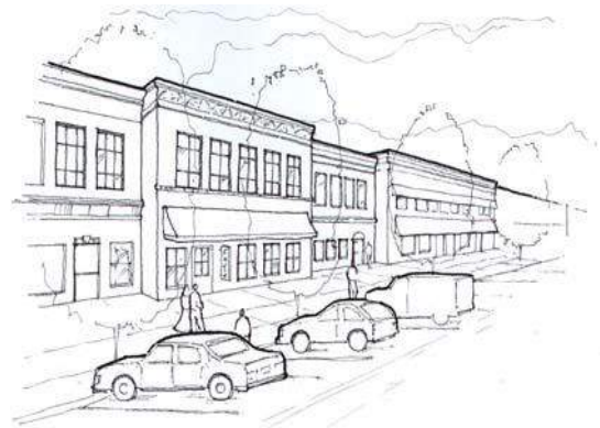
Figure 8-2. Long building facades should use variations in building mass while still presenting a consistent streetscape.
